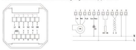
LCF Touch Modbus - Manual mode wiring diagram for 2-pipe fan coil
