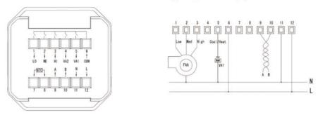
LCF Touch Modbus - Auto change-over mode Heating/Cooling wiring diagram for 4-pipe fan coil
